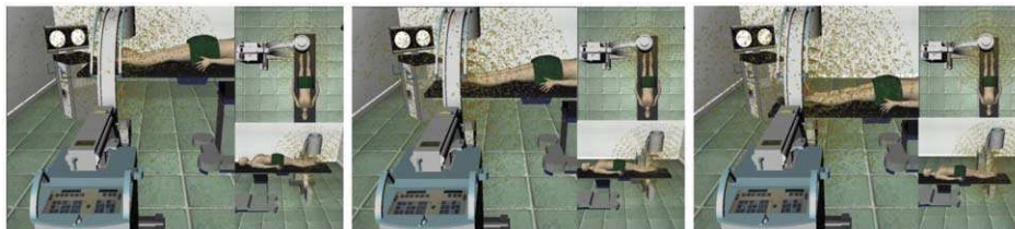
Figure 3. Visualization of the GEANT4 calculations in the 3D scene of the virtX system for different C-arm/table adjustments (5000 photons, 9 detector spheres)
